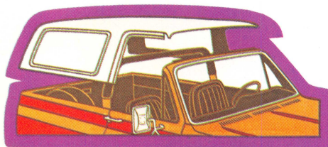
The closed hard top Jimmy model comes complete with roll bar and tailgate with manually operated dropglass. Top may be removed as shown.
