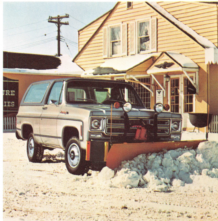
Power take-off with either full-time or conventional four-wheel-drive provides power for utility accessories including rotary brooms and snowplows.
